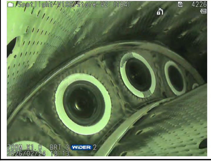
Fuel Nozzle Swirler Ring with TBC loss - Serviceable
