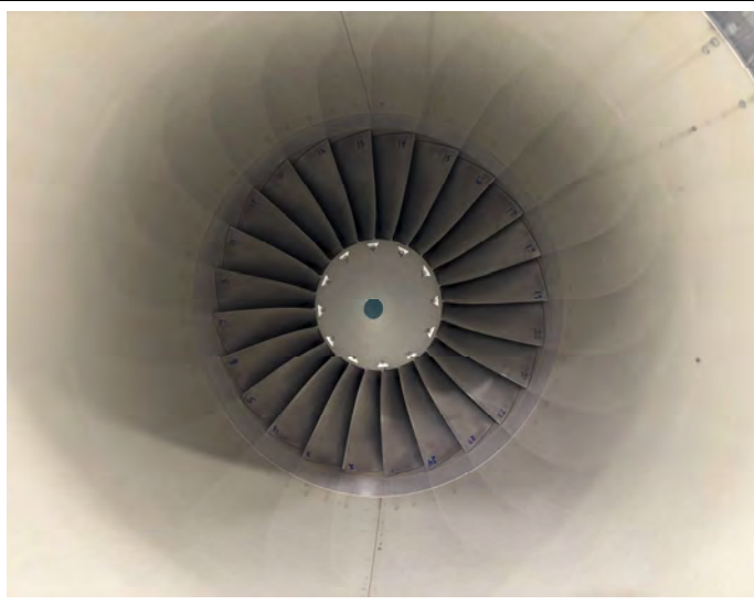
Fan Assembly - Unserviceable (FOD)
