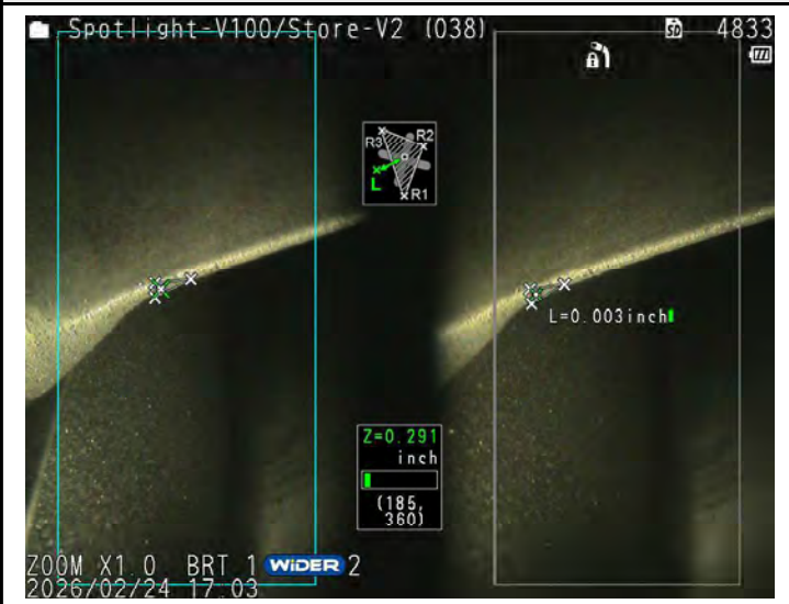
Fuel Nozzle Swirler Ring with TBC loss - Serviceable
