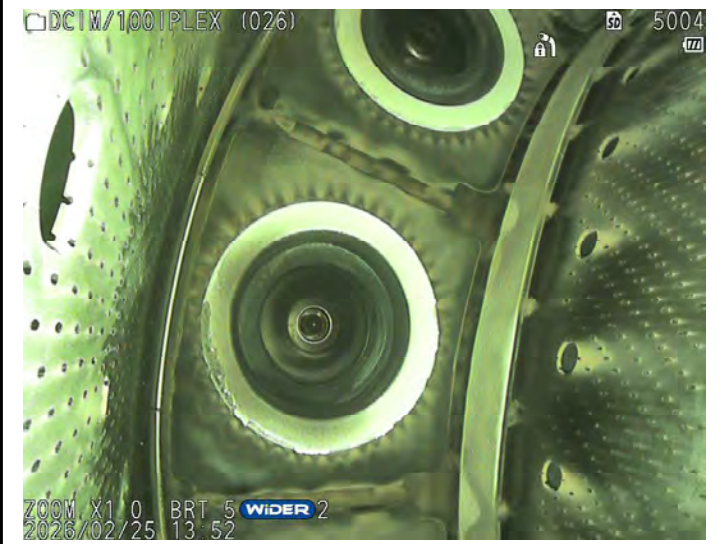
Outer Liner Crack - Serviceable
