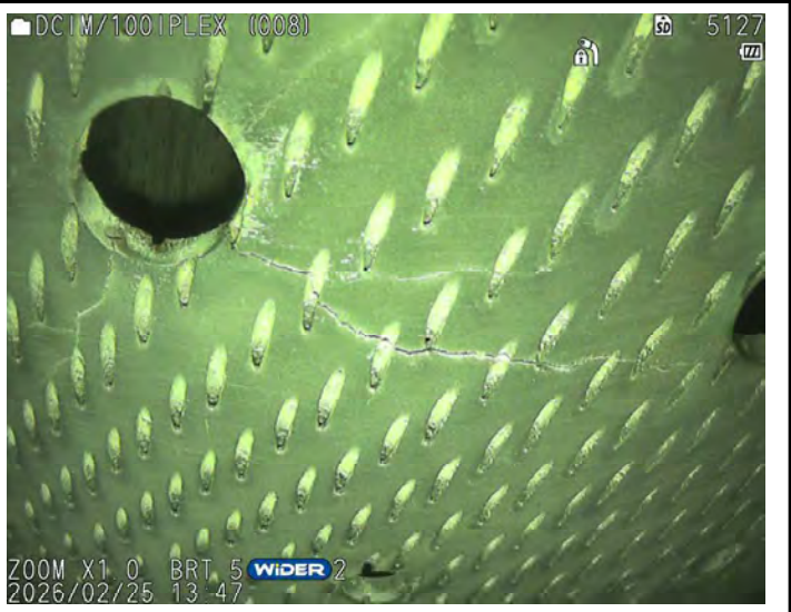
Outer Liner Crack - Serviceable
